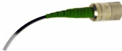
Figure 3: Photo of the fiber-optic accelerations sensor. The diameter of the aluminum tube is 11 mm. The cable that leaves the sensor is an optical fiber, not a copper wire.
