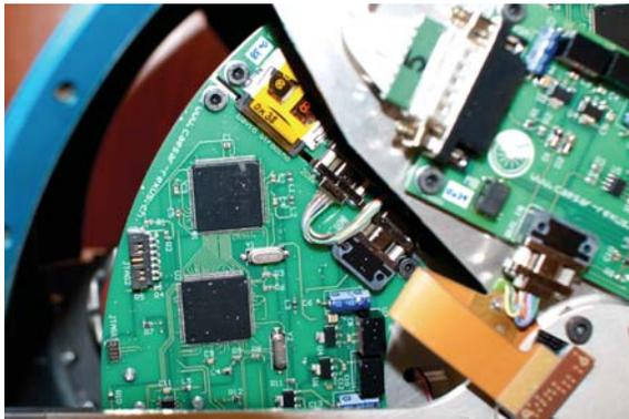
Figure 5. Metallic particles on the experiment PCB
