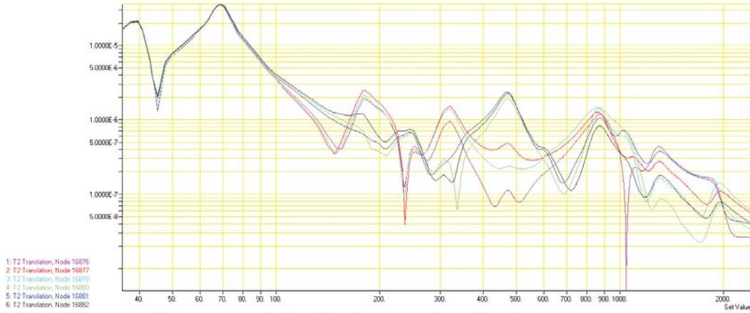
Figure 12. Modal Frequency Response Analysis – Displacement along Y-axis
