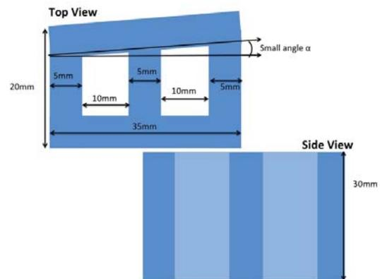
Figure 4. Experimental Cell Design
