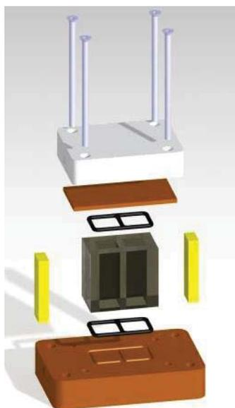
Figure 3. Experimental Cell Design
