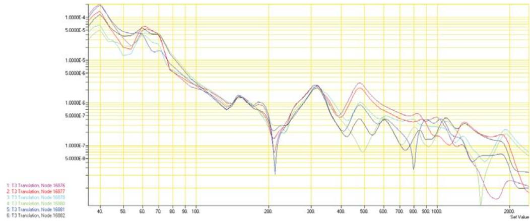
Figure 13. Modal Frequency Response Analysis – Displacement along Z-axis
