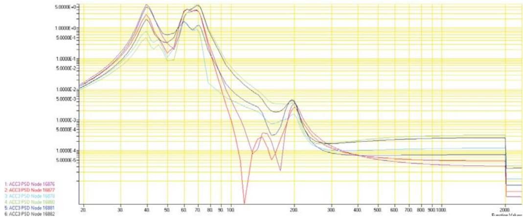
Figure 16. Random Response Analysis – Accelerations along Z-axis.
