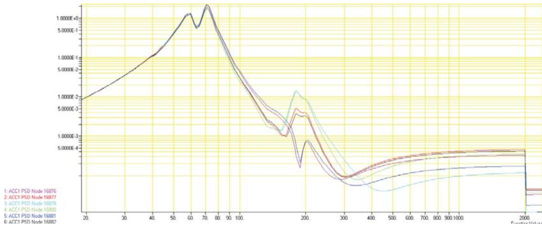
Figure 14. Random Response Analysis – Accelerations along X-axis
