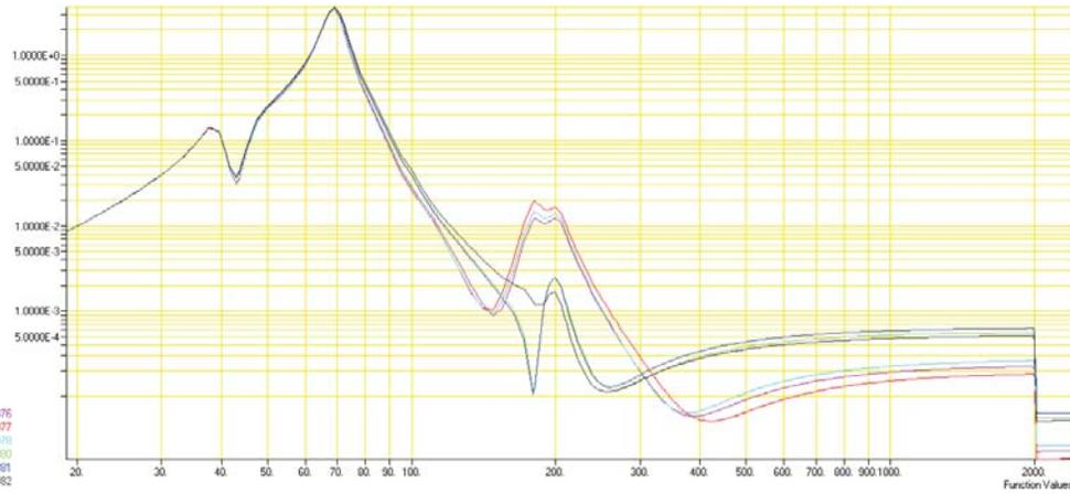
Figure 15. Random Response Analysis – Accelerations along Y-axis
