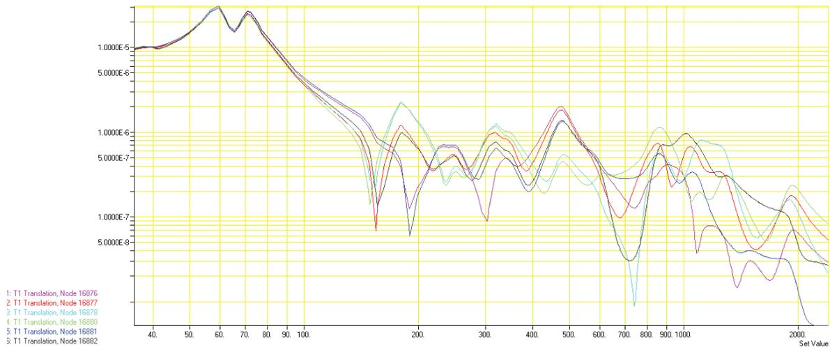
Figure 11. Modal Frequency Response Analysis – Displacement along X-axis.
