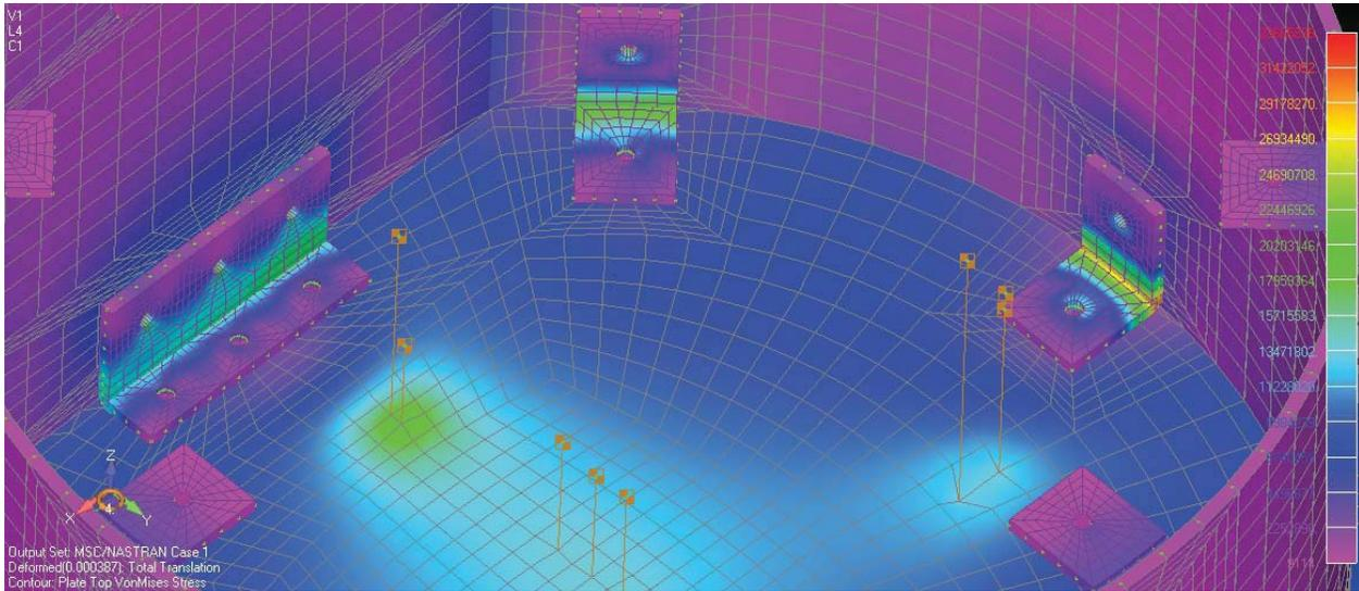
Figure 9. Closeup of CWIS module without top plate (Contours of Von Mises stress)
