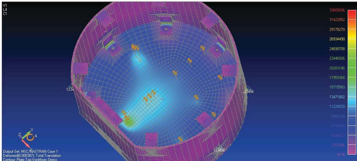
Figure 8. FEM of CWIS module without top plate (Contours of Von Mises stress)
