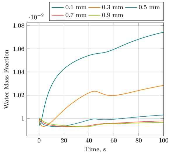
Figure 10. Water mass fraction over time in ground gravity condition at different distances from the hot wall
