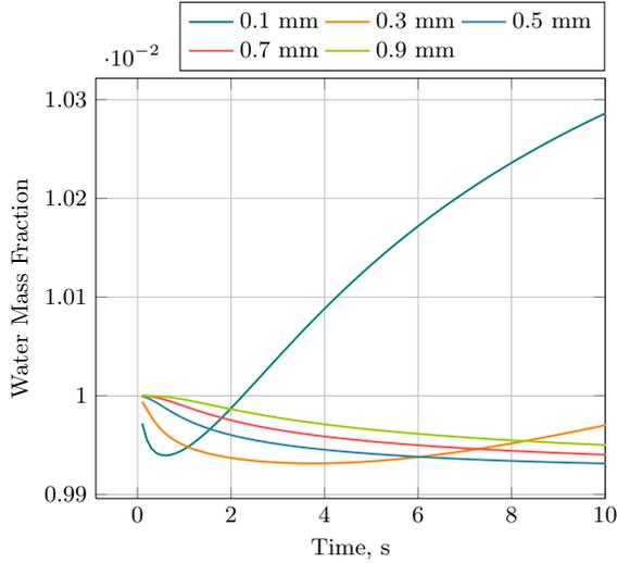
Figure 6. Water mass fraction over time in no gravity condition, 10 K temperature difference at different distances from the hot wall
