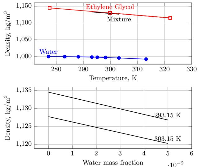
Figure 3. Density of the mixture vs temperature and water mass fraction. The trend of water density over temperature is assumed to be linear within the temperature range of interest. The mixture density is evaluated considering a water mass fraction of 0.01.
