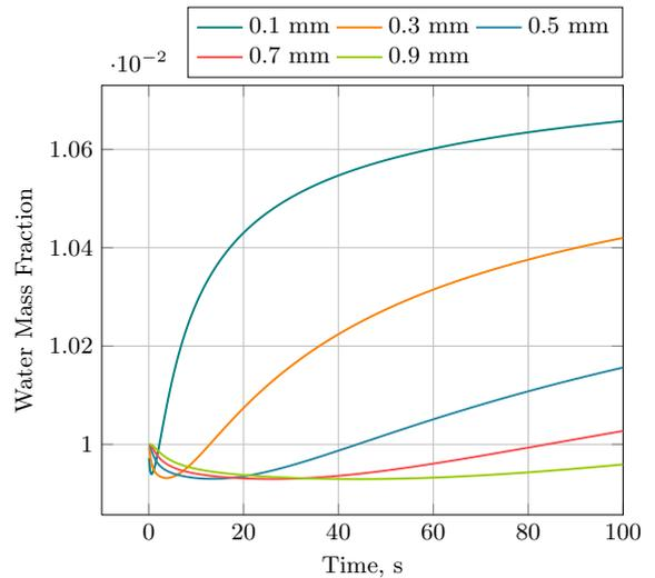
Figure 5. Water mass fraction over time in no gravity condition, 10 K temperature difference at different distances from the hot wall
