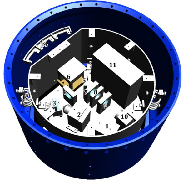
Figure 2. Experiment: 1. Laser, 2. Microscopic Objective, 3. Mirror, 4. Collimating Lens, 5. Beam Splitter, 6. Liquid Cell, 7. Spherical Lens, 8. First Cylindrical Lens, 9. Second Cylindrical Lens, 10. Camera, 11. Electronics, 12. Damping Springs, 14. Feed Through Cable Bracket
