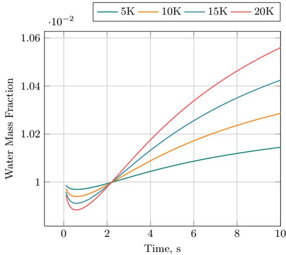
Figure 8. Water mass fraction over time in 0-gravity condition, at different temperature differences and at 0.1 mm from the hot wall
