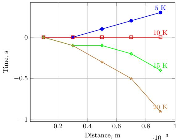
Figure 9. Time difference between reference case and others at various temperature differences: 5 K, 15 K, 20 K
