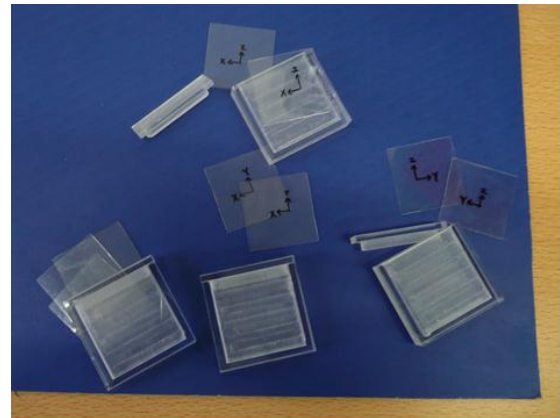
Figure 4. Holders and TASTRAK SSNTDs used in the balloon experiments.
