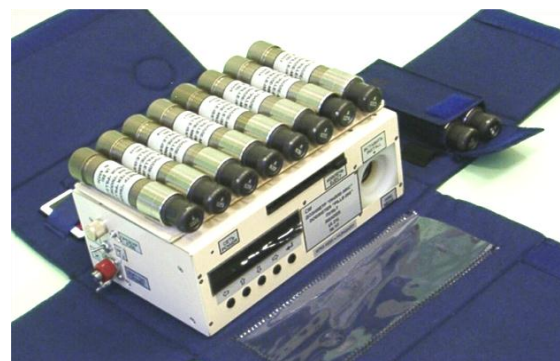
Figure 3. The Pille TL dosimeter system in its transporting case (reader and ten dosimeters).
