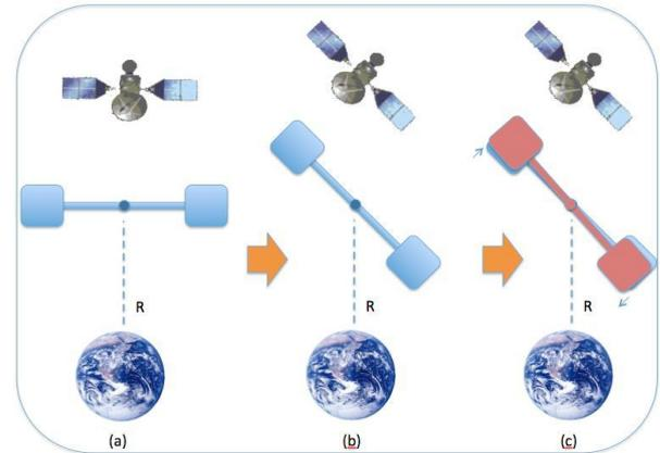
Figure 1. Diagram showing effect of the gravity gradient on an elongated proof mass. (a) the proof mass inside the satellite is perpendicular to the Earth. Both sides of the mass being the same distance from the Earth, there is no detectable effect. If the satellite rotates by a given amount (b), the mass inside also rotates. Since now one side is closer to the Earth and sees more gravity (c), the GGT will produce a displacement
