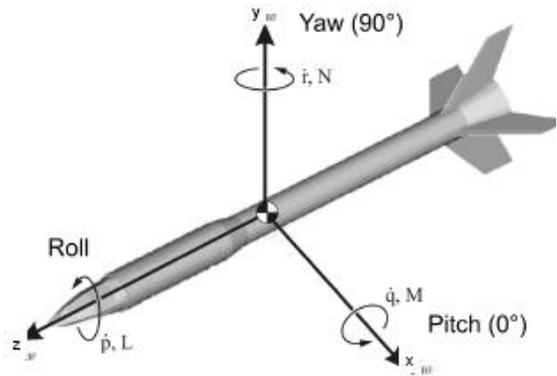
Figure 3. REXUS body frame coordinate system. [4]
