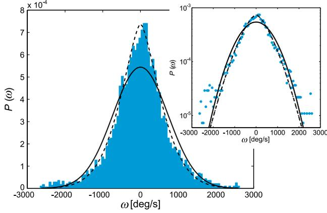
FIG. 4 (color online). Rotational velocity distribution at Excitation (1). Solid line: Gaussian with the parameters for  $\omega$  from Table I, dashed curve:  $P(\omega) = 0.00074 \exp\{-(|\omega - \mu_\omega|/748.5 \text{ deg/s})^{1.5}\}$ .
