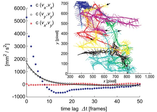
FIG. 2 (color online). Temporal autocorrelation and cross correlation of the translational velocities in the direct excitation direction ( $x$ ) in the indirectly excited direction ( $y$ ) at Excitation (1). The inset shows exemplary rod trajectories over 101 frames, arrows indicate the beginning.
