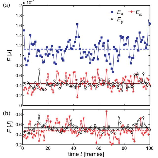
FIG. 5 (color online). Energies  $E(t)$  in the observed degrees of freedom for the 30 Hz (a) and 20 Hz (b) excitations. Horizontal lines reflect the time averages from Table I. For the 20 Hz excitation, the  $E_x$  curve is qualitatively similar to that for 30 Hz in (a).
