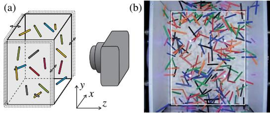
FIG. 1 (color online). (a) Schematic experimental setup and selected coordinate system: container with 3 moveable walls agitated by voice-coil actuators, width: 8.5 cm, height 10 cm, depth 6.3 cm, top camera not shown; (b) freeze frame of the granular gas of 250 colored rods excited by shaking side walls (30 Hz) in microgravity. The white box indicates the region selected for statistical evaluation. See Supplemental Material [32] for movies of the granular gas.
