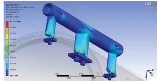
Figure 7. The results of a vibration simulation
