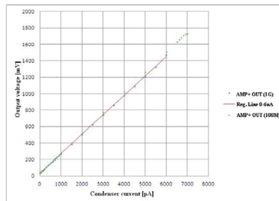
Figure 11. Positive amplifier, transfer characteristic
