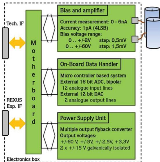
Figure 9. Gekko electronics, block scheme
