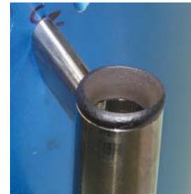
Figure 16. Melted plastic insulation ring
