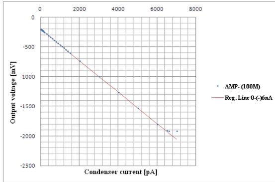
Figure 12. Negative amplifier, transfer characteristic
