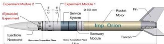
Figure 5. A standard REXUS configuration [2]
