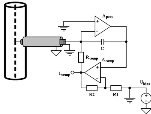
Figure 10. Current measurement method
