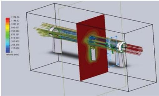
Figure 8. The trajectories of the airflow inside and around the condensers
