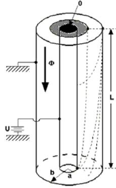
Figure 2. Gerdien condenser, working principle [3]
