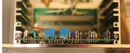
Figure 14. PSU PCB in the electronics box
