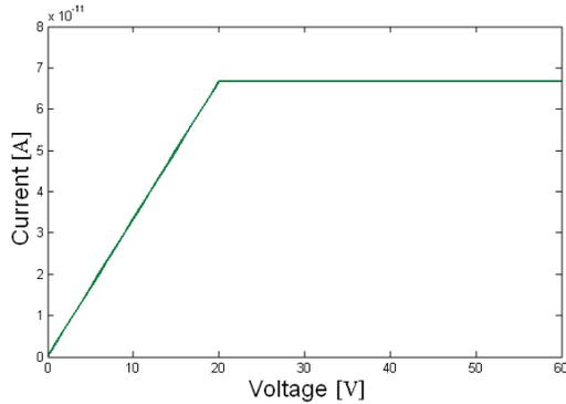
Figure 3. Ideal voltage-current characteristic
