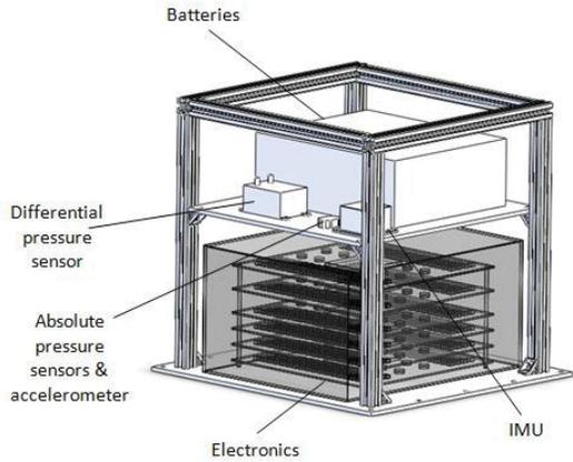
Figure 2. Internal components of MISSUS experiment
