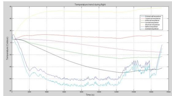
Figure 8. Temperature of MISSUS components
