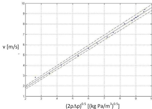
Figure 13. Pitot tube calibration curve
