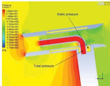
Figure 6. Pitot tube, CFD analysis
