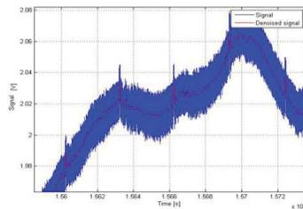
Figure 15. Temperature sensor signal before and after de-noising
