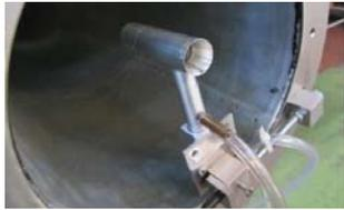
Figure 12. Pitot tube calibration set-up
