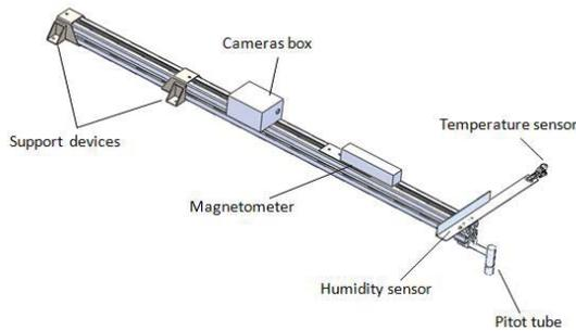
Figure 3. External components of MISSUS experiment
