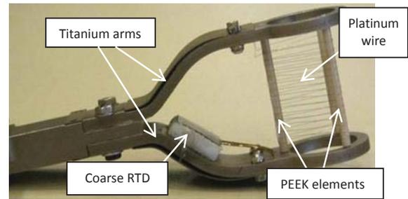
Figure 4. Innovative temperature sensor
