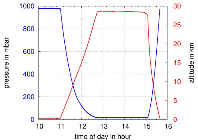
Figure 2. BEXUS 14 altitude and pressure time profile [4].
