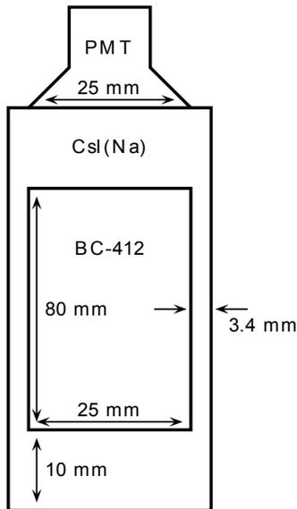
Figure 1. Schematic of the Phoswich Instrument for Neutrons and Gammas [3].
