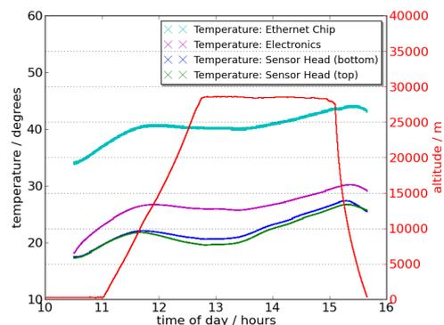
Figure 3. Thermal behaviour of the experiment during the flight.
