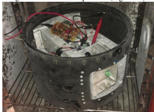
Figure 13: Freezing condensation on experiment when thermal chamber door was opened at -10C.
