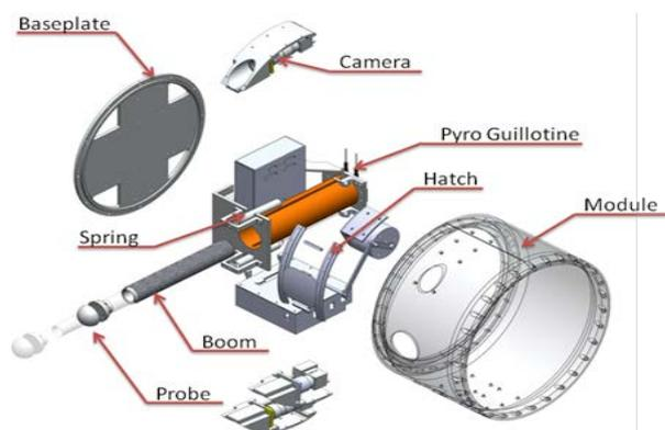
Figure 3: An exploded view of the experiment module with important components labelled.
