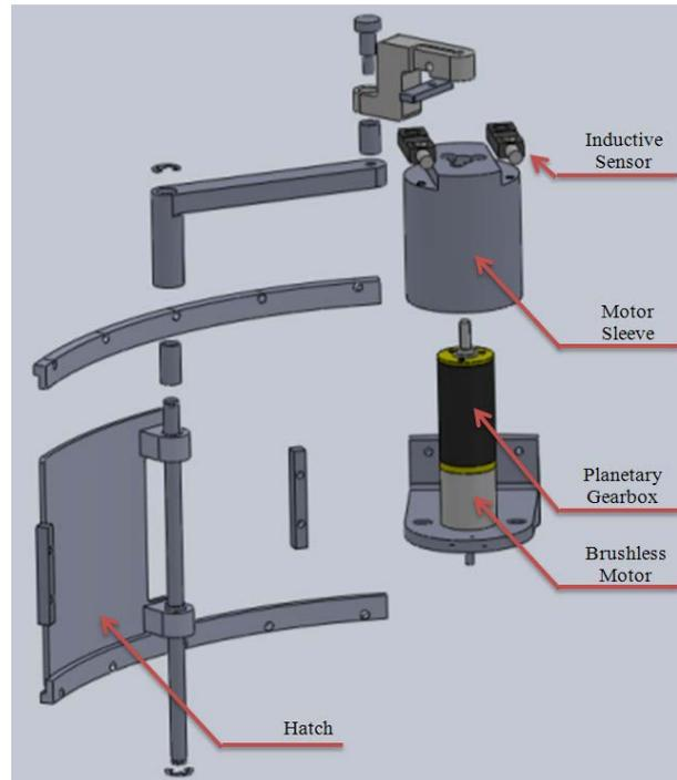
Figure 4: Exploded view of the experiment hatch assembly
