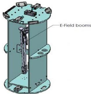
Figure 1: Typical folded boom sections for E-Field probes [2].
