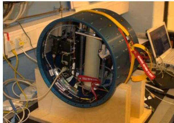
Figure 5: The Telescope module ready for final payload integration
