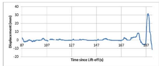
Figure 9: Displacement of the distal end of the boom in an axis parallel to a plane between the payload X-axis and Y-axis during the first 105 seconds after boom deployment.
