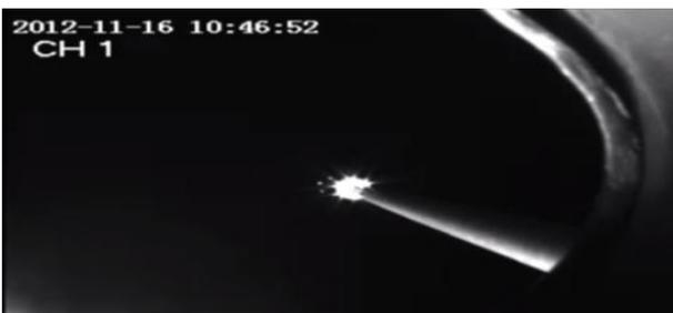
Figure 7: The telescopic boom deployed from the experiment module 12 seconds after boom deployment.
