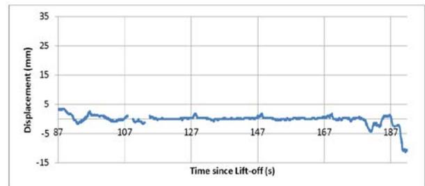
Figure 10: Displacement of the distal end of the boom in an axis parallel to the payload Z-axis during the first 105 seconds after boom deployment.
