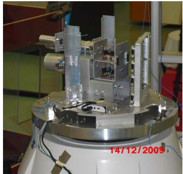
Figure 7 – BUGS experiment vibration test at the ESTEC/ESA
