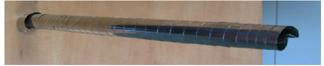
Figure 2 – Tape coil spring employed for boom prototype development.
