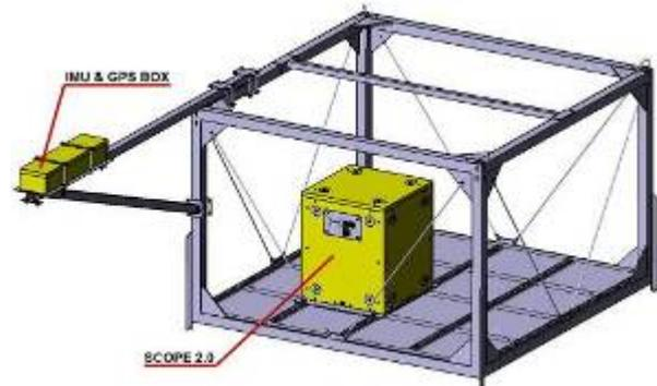
Figure 8. Position of the prototype of proposed camera stabilization and control system (SCOPE) in the BEXUS 11 gondola (IMU/GPS box is located on a boom)
