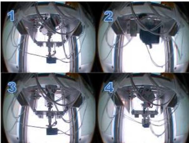
Figure 16. Pre-programmed test sequence of motion performed at the height of 16 000 m (pressure: 93mbar, external temperature: -53 °C)
