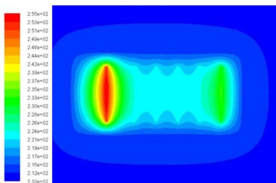
Figure 12. Thermal analysis of the electronic box
