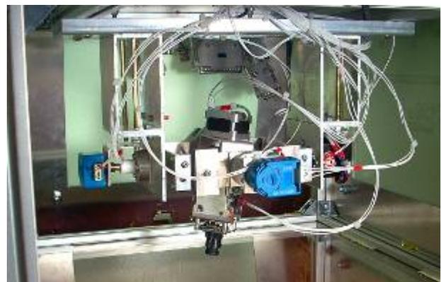
Figure 10. Prototypic realization of Platform Orientation Mechanism (POM) for BEXUS 11 flight
