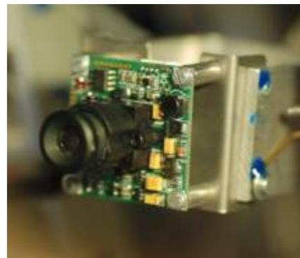
Figure 6. Video camera mounted on the POM
