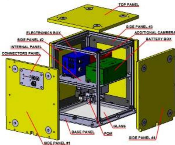
Figure 7. Schematic view of the prototypic realization of the camera stabilization and control system
