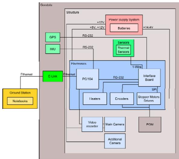
Figure 2. Overview of the camera stabilization and control system
