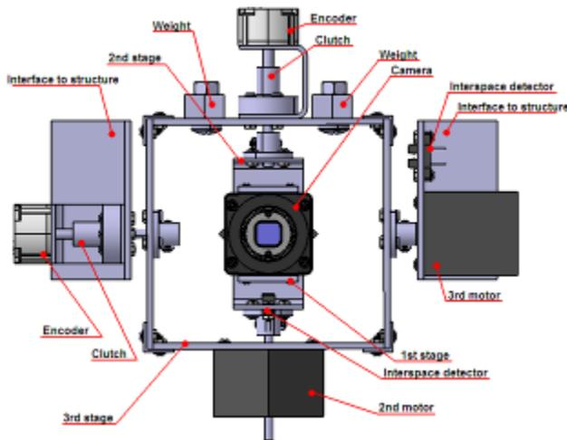
Figure 9. Schematic view of the Platform Orientation Mechanism (POM)
