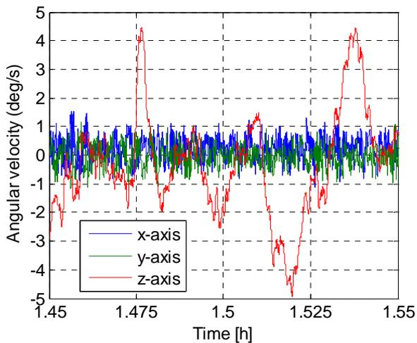
Figure 1. Angular velocities of the stratospheric balloon gondola during ascent (based on Low.Co.I.N.S. data obtained during BEXUS 6 flight in 2008)
