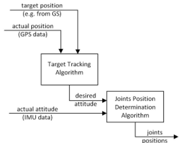
Figure 3. Control algorithms for tracking ground targets
