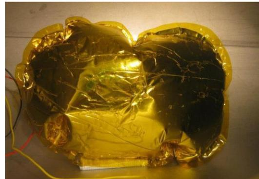
**Figure 2: Inflated cell in vacuum chamber**
