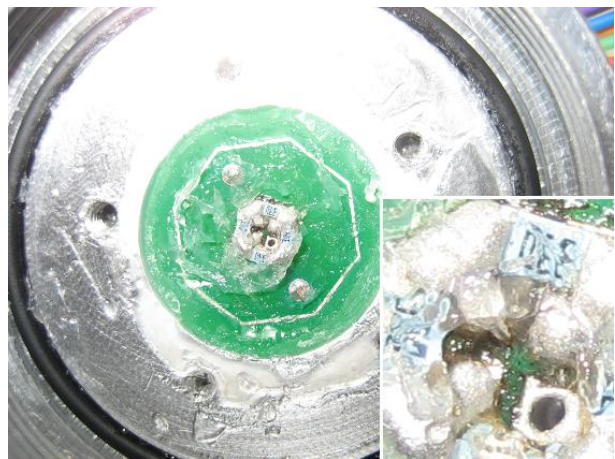
Figure 11. Looking at the pressure side of the CO_2 cartridge lid after the valve failure. The four valve resistors are thermaly insulated by grease and a PEEK plate (removed in figure).
