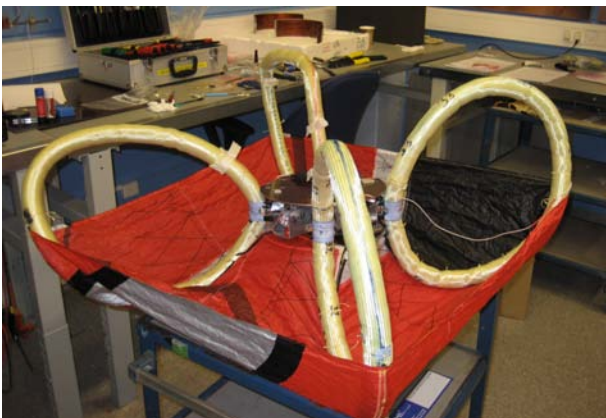
Figure 1. LAPLander showing the correct ballute geometry.
