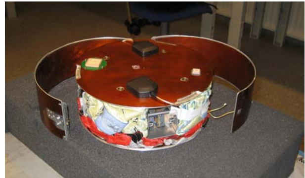
Figure 2. LAPLander with the hatch and the rope cutting mechanism (cutter dummy).
