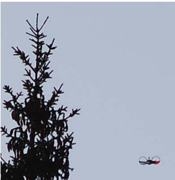
Figure 5. A scale 1:1 model with rigid airbags in free flight from a helicopter at 1500 m, seen from a distance.
