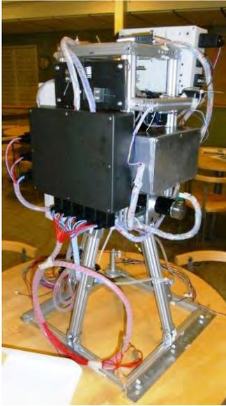
Figure 3. Photograph of the assembled reel. SMRT MAIN Payload with the insulation removed and the electronics boxes distributed around the frame
