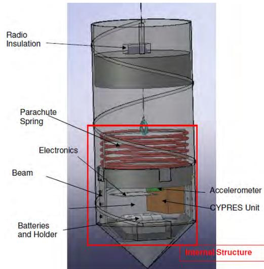
Figure 6. The positioning of key mechanical and electronic systems within the FISH
