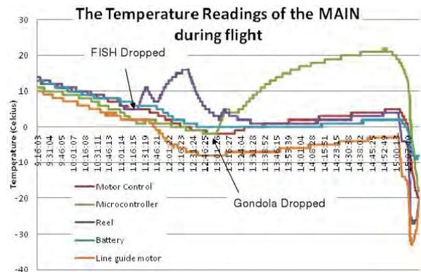
Figure 12. Temperature readings of the MAIN Payload during the flight
