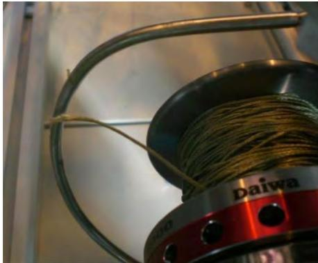
Figure 10. Close-up of the broken line as it was stuck on the bail when recovered
