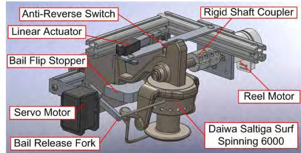
Figure 4. Bail Mechanism of the MAIN Payload
