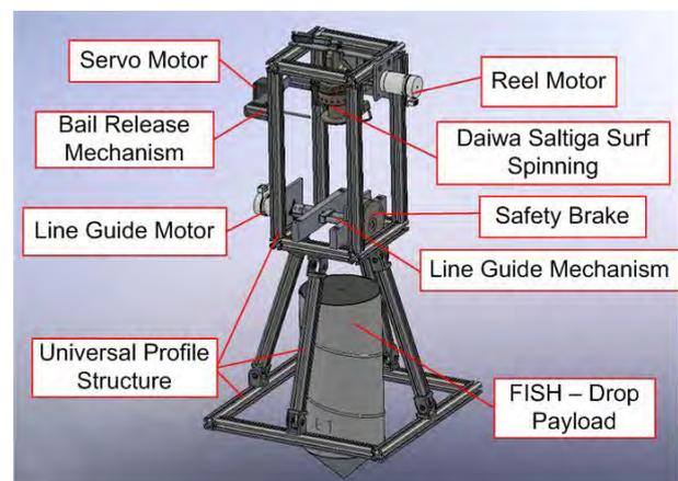
Figure 2. Mechanical System
