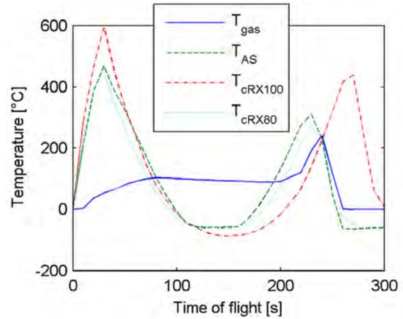
Figure 5. Calculated gas and probe surface temperatures as a function of the time of flight compared to the data recorded during the real flight
