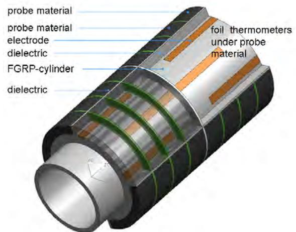
Figure 6. Probe Assembly
