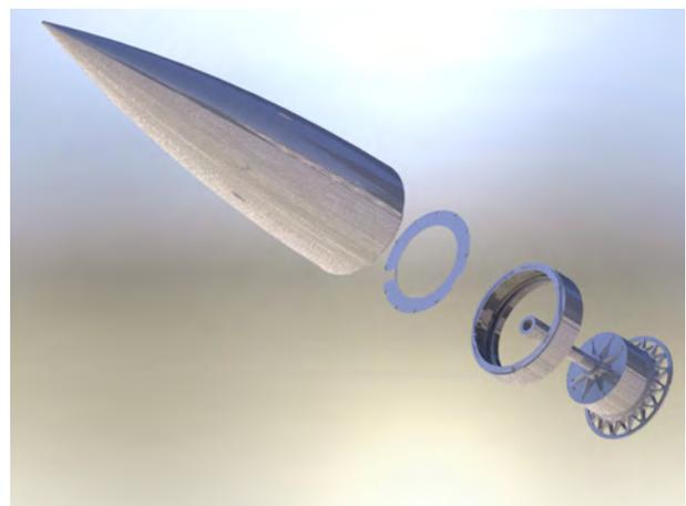
Figure 1. REXUS nosecone section
