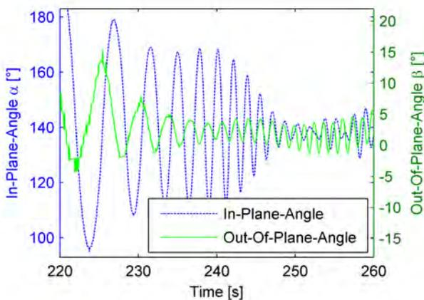
Figure 12. Coupling of  $\alpha$  and  $\beta$  at  $t = 220$  s . . . 260s
