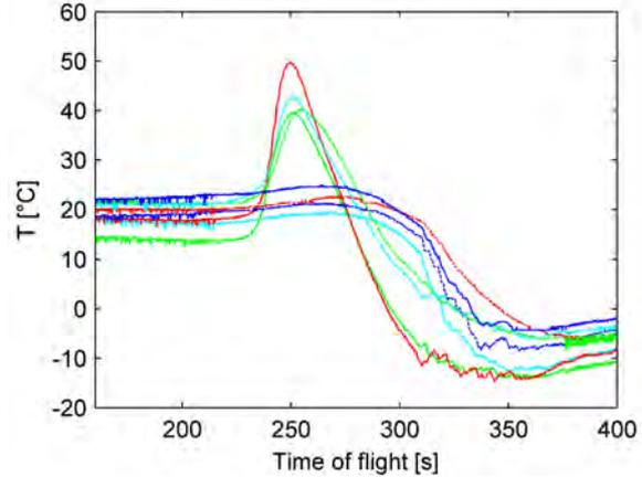
Figure 13. Temperatures measured under the 8 probe segments during reentry phase.
