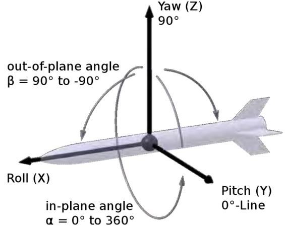
Figure 3. Body Frame Coordinate System
