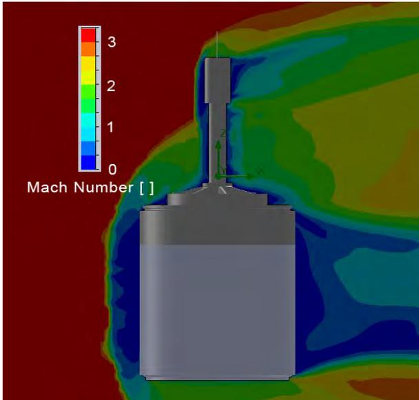
Figure 4. Map of the Mach number around the experiment module at an altitude of 20 km
