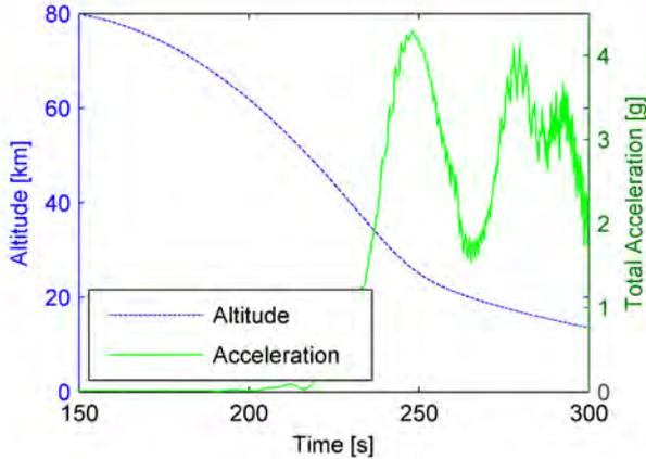
Figure 11. Altitude and total acceleration  $a_{total}$  at  $t = 150$  s . . . 300s
