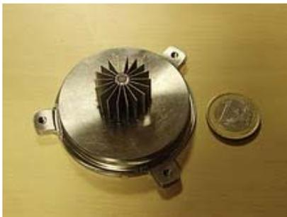
Figure 1. sponge PMD device mounted on its titanium base.
