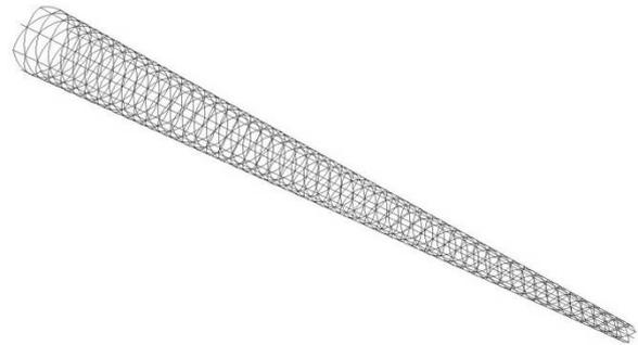
*Figure 10. IsoGrid Boom Structure*
