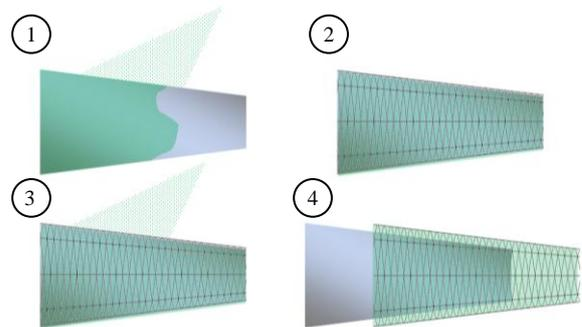
*Figure 11. Manufacturing concept utilising mandrells and sprayable membrane technology*
