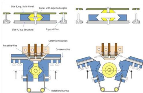
Figure 3. Sketch of HDRM and Functional Principle
