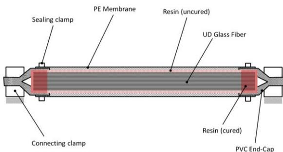
Figure 1. Detailed design of a FOCUS composite beam
