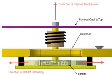
Figure 4. Arrangement of Release- and Push-Hardware
