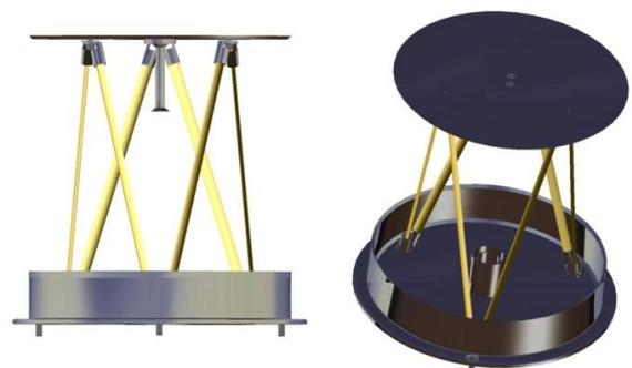
Figure 2. Deployable composite structure integrated with the Storage Container
