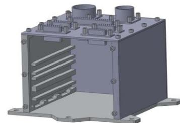
Figure 5. The Electronic Box without the printed circuit boards.
