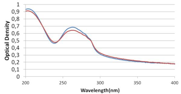
Figure 11. Example of the OD decrease of an uracil sample. Blue: before flight, red: after flight data
