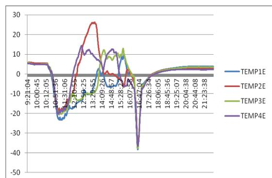
Figure 8. Thermal behaviour of the four optical boxes Temperature shown was measured outside the MLI foil.
