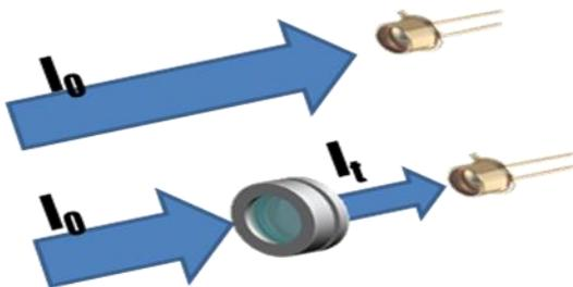
Figure 3. The scheme of OD measurement in the BioDos experiment
