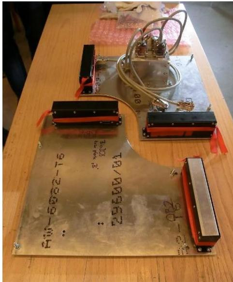
Figure 6. Experiment units: four optical boxes and the electronics box mounted on the base plates
