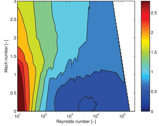
Figure 2. Drag coefficient of the sphere.
