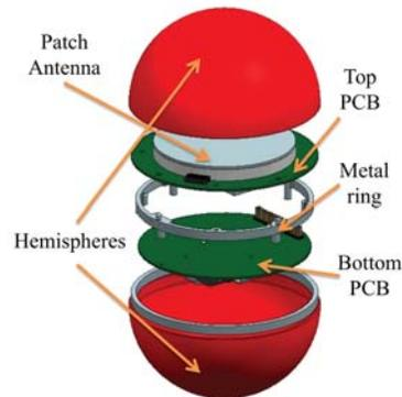
Figure 9. Free Falling Unit explosion view with hemispheres, top PCB, bottom PCB, metal ring and patch antenna.
