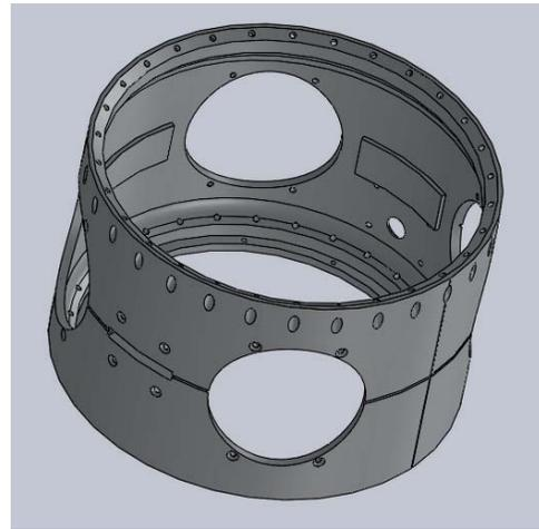
Figure 5. Modified rocket cylinder with four openings, cable groove and additional components.
