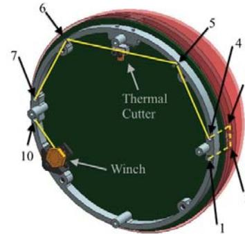
Figure 12. Nylon string securing the upper hemisphere to the PCB assembly.
