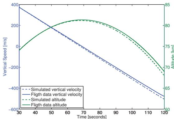
Figure 18. Altitude and vertical velocity of the FFU during free fall from flight data and simulation.
