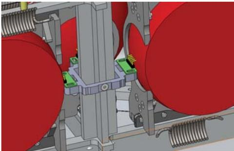
Figure 7. Position of the five pins umbilical connector.
