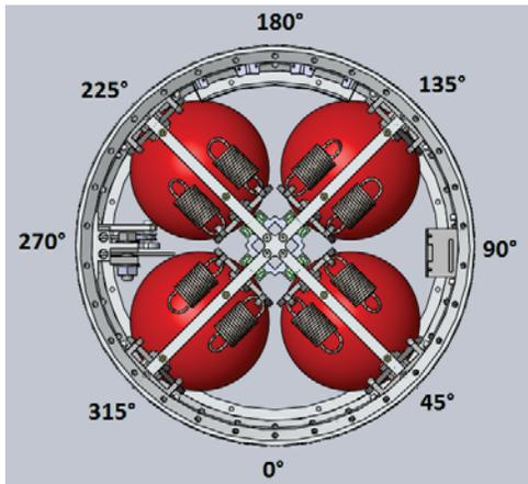
Figure 4. Rocket Mounted Unit (RMU). Openings for the ejection of the FFUs are positioned at 45°, 135°, 225° and 315°. Pyrocutter module is positioned at 270° and onboard camera is at 90°.
