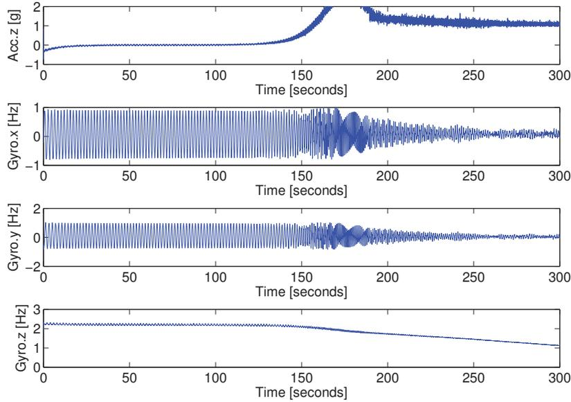
Figure 14. Inertial sensor data of a flight FFU: acceleration in z direction and x, y and z component of the angular rate.
