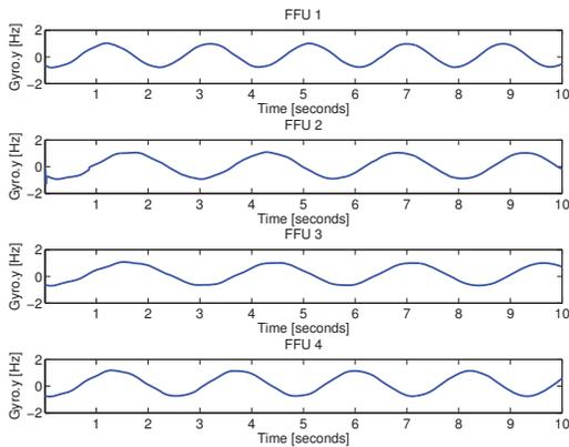
Figure 15. Angular rate around y-axis for the first 10 seconds after ejection.
