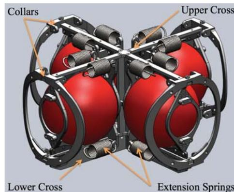
Figure 6. Ejection system with upper and lower crosses, collars and extension springs
