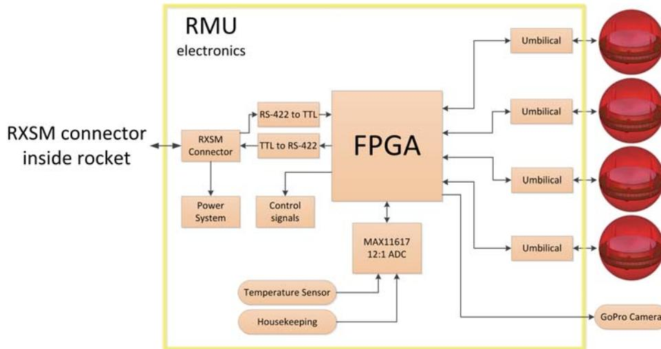
Figure 8. Conceptual diagram of the RMU electronic system.
