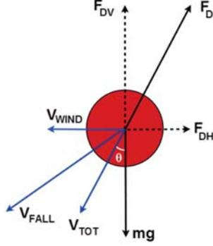
Figure 1. Forces acting on the probe during free fall.
