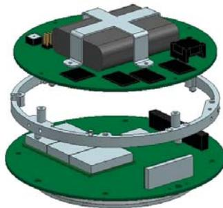
Figure 11. PCB assembly with all large electrical components, upside-down.
