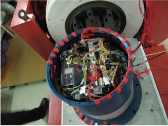
*Fig 13 Redemption module at vibration test in ZARM*
