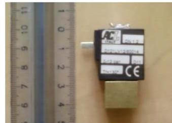
*Fig.6 Electrovalves provided by ACL*
