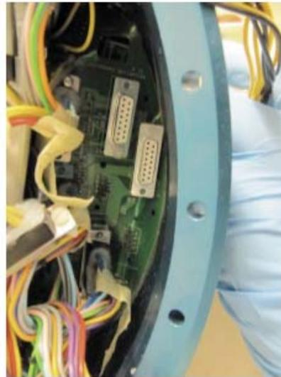
*Fig 18 Investigation after the crash: PCB damaged*
