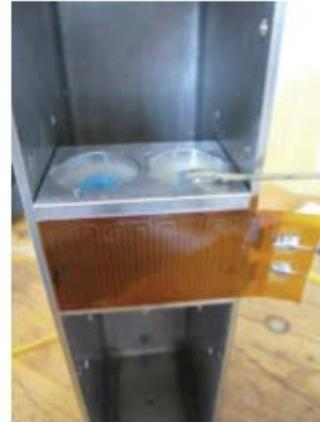
Fig. 9 Thermal control system based on kapton film
