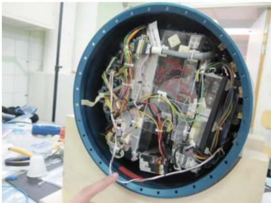
Fig 11 Redemption module fully integrated in the skin
