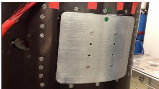
Figure 4: Hatch Slip after Vibration Testing
