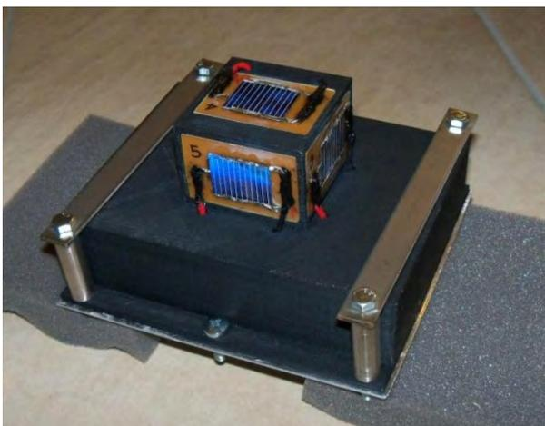
Figure 2. Sun sensor in flight configuration
