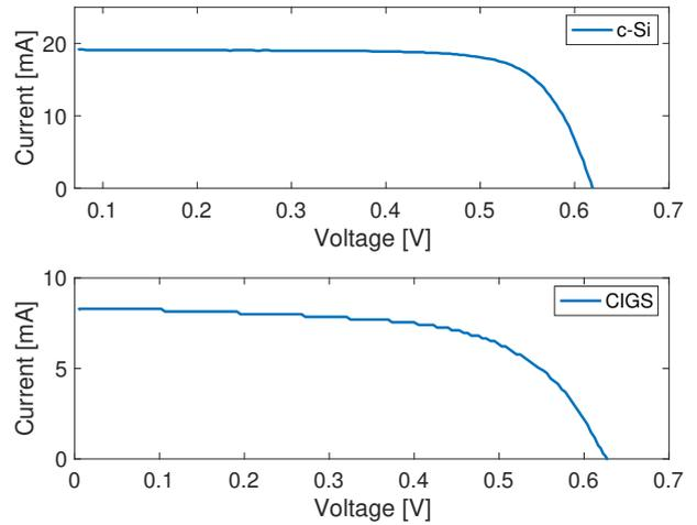
Figure 4: Example of in-flight IV characterization of c-Si and CIGS solar cells.
