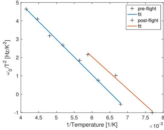
Figure 9: Arrhenius plot for a CIGS solar cell before and after exposure.
