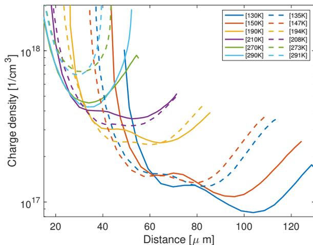
Figure 11: Doping profile before (dashed) and after (solid) flight for a CIGS solar cell.
