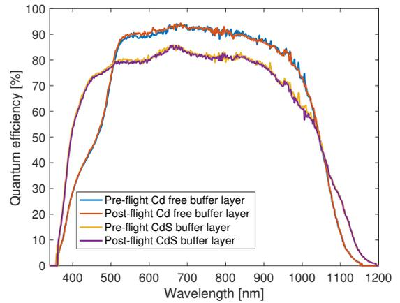
Figure 7: Quantum efficiency of CIGS solar cells before and after flight.
