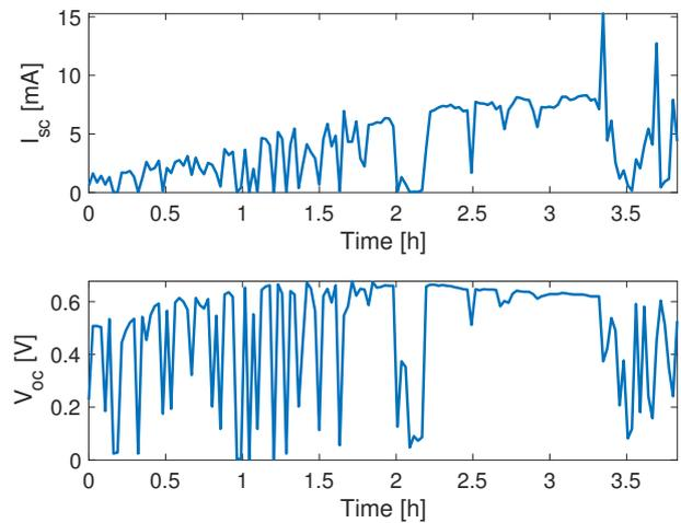
Figure 5: Variation of  $V_{oc}$  and  $I_{sc}$  for CIGS solar cells during flight.
