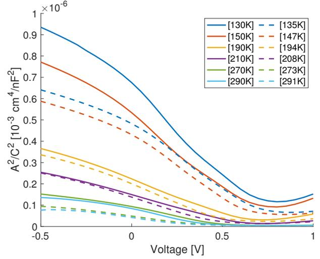
Figure 10: Mott-Schottky plot of a CIGS solar cell. The dashed line shows the pre-flight characterization and the solid line the post-flight characterization. The area of the CIGS was  $A = 5 \text{ mm}^2$ . The frequency of the CVT measurement was 100 kHz.
