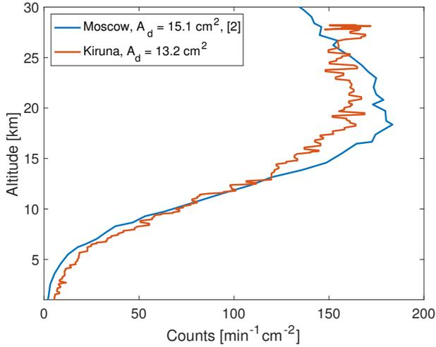
Figure 2: Radiation counts/min  $\text{cm}^2$  for different altitudes during ascent compared to similar measurements by [2].
