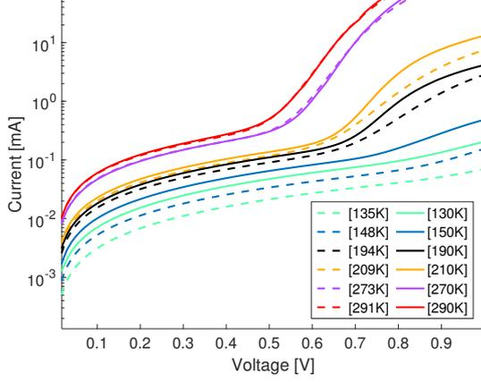
Figure 8: IVT characterization of a CIGS solar cell. Pre-flight characterization is the dashed line and the post-flight characterization is the solid line.
