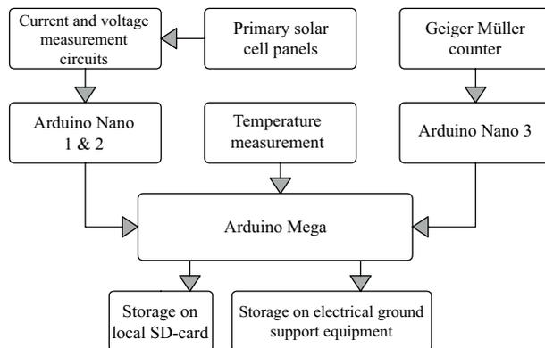
Figure 1: Schematic of the measuring device and the data transfer.
