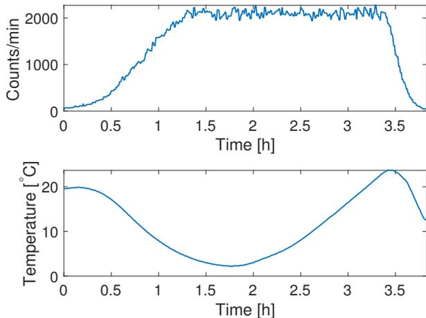
Figure 3: Radiation counts and temperature inside the electronics box as a function of flight time. The total number of counts during the flight were 349614. The energy deposited in a  $5 \times 5$  cm solar cell panel was  $1.3243 \cdot 10^{15}$  eV = 0.2 mJ.
