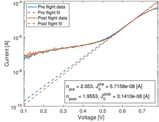
Figure 6: High precision IV characterization of CIGS before and after flight. From the fit of the linear region in the semilog plot the ideality parameter and the reverse saturation current can be extracted.
